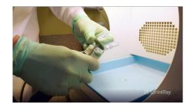
Use low RPM with a Scotch Brite wheel or carbide bur to remove any stumps left over from supports. Use 10,000-12,000 RPM.
