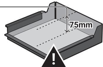
Do not try to close the curing drawer if models exceed the height limit; this may permanently damage ProCure 2.
