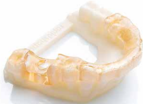
2x surgical guides, printed in ~ 15 minutes
