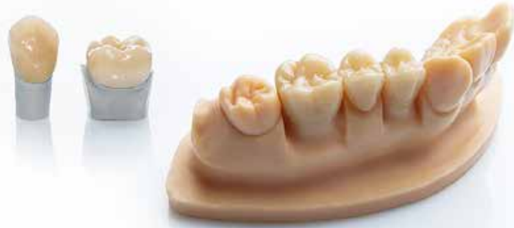
28x crown & bridge units, printed in ~ 15 minutes
